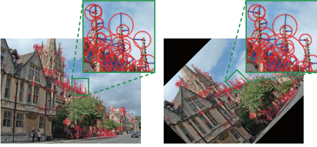
Fig. 6. Examples of detected keypoints by Cascaded FAST.
