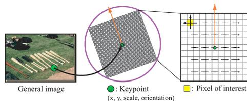
Figure 1: Gradient extraction in a local patch.
