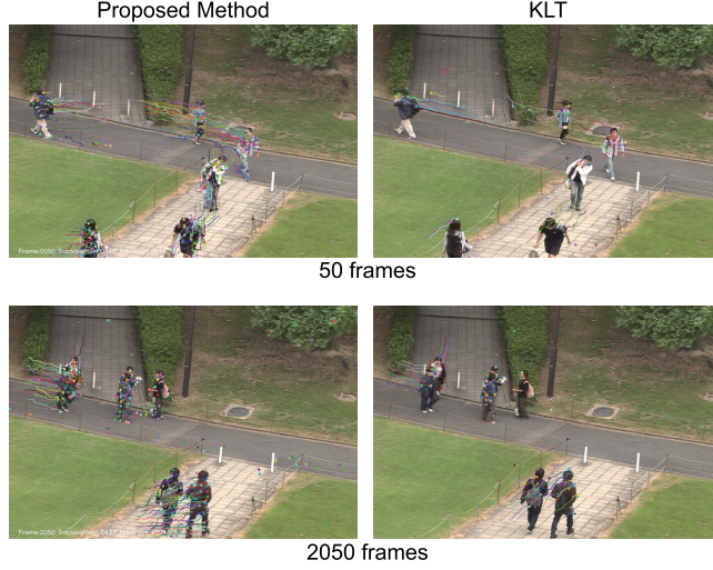
Fig. 7. Examples of Feature Point Tracking for Images of Pedestrians
