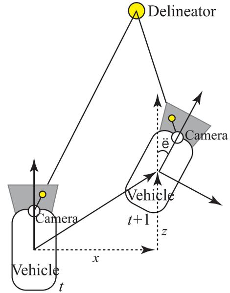
Fig. 5. Stereo vision between consecutive frames using data.
