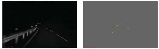
Fig. 9. Example of detection of delineators.
