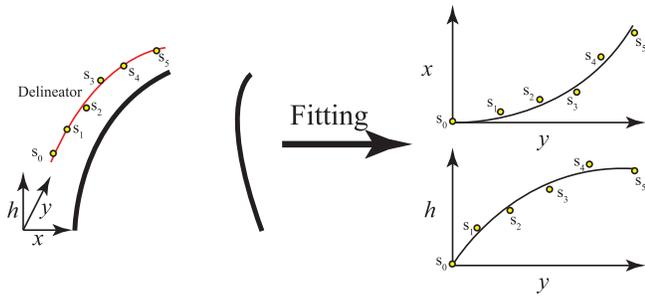
Fig. 8. Clothoid curve and cubic function are applied to 3D position of delineator.
