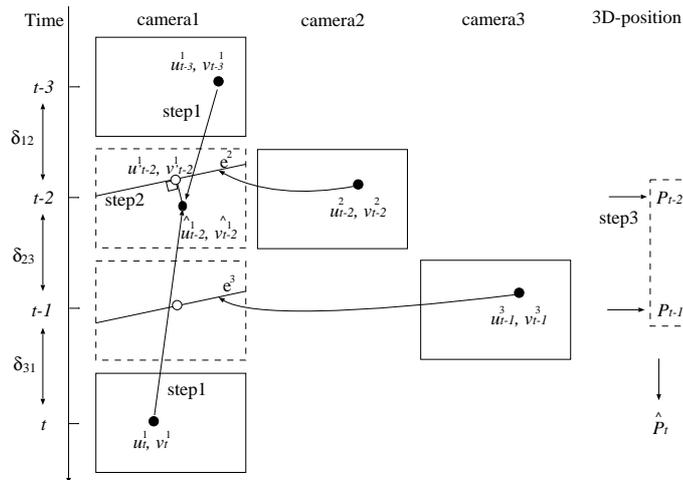
Fig. 2. Proposed calculation method of corresponding position
