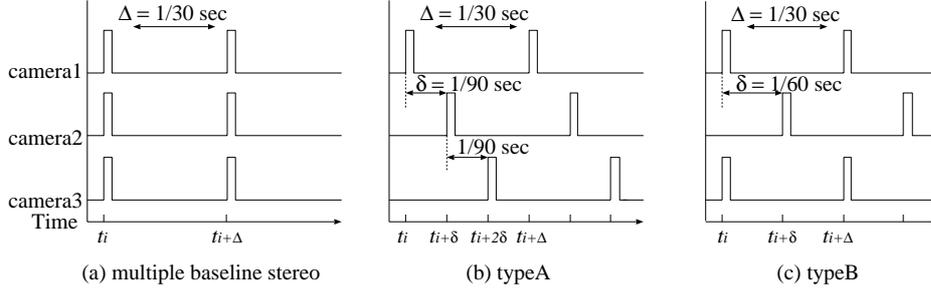
**Fig. 1.** Possible two combinations of shutter timing
