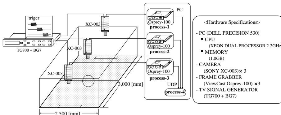
Fig. 5. Hardware specifications
