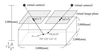
Fig. 5. Virtual camera placement in simulation experiment
