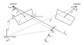
Fig. 4. Constraints in estimating 3D position
