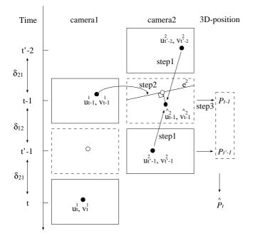
Fig. 3. Proposed calculation method of corresponding position
