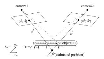
Fig. 2. Errors occured in stereo vision with time delay
