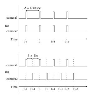
Fig. 1. Synchronized and unsynchronized camera timing
