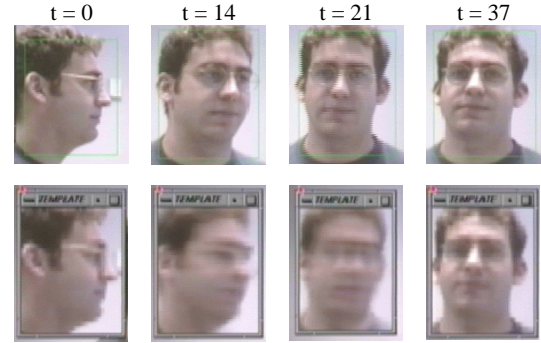
Figure 8. The IIR lter. As the image changes from a face in prole to a frontal view, the template is updated using an IIR. If the image is stable for some time, the template also remains stable.
